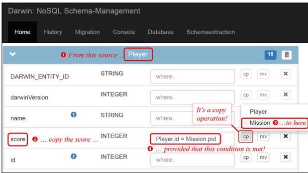
Fig. 4: Declaring a schema evolution operation using the graphical interface of Darwin.
