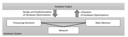
Fig. 1: Overview of Hardware/Software Co-Design for Database Engines.
