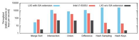
Fig. 10: Throughput for different operations.
