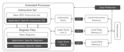
Fig. 4: The Tensilica LX5 Processor and the surrounding components have been extended by the features highlighted by a gray box.
